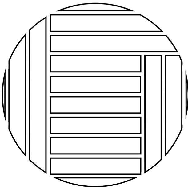
FIGURE 4: The sawing-for-grade cutting pattern used to saw the pruned butt logs into 40-mm thick random-width boards.
